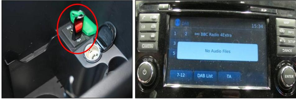
7 Press and hold the 'Setup' button and then turn the 'Enter' button a half turn anti-clockwise, then a half turn clockwise, then a half turn anti-clockwise. The 'Service Menu' will then appear. Release the 'Setup' button.
