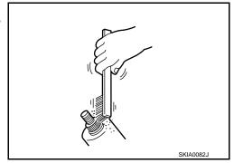
When installing the wiper arm, install so that it is within the standard. For the standard, refer to WW\_ 80, "WIPER ARM: Adjustment".
