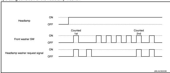
Operate by front washer switch at the first time
