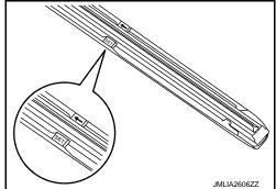
Pass through pawl of wiper blade in the groove of wiper refill. NOTE:
