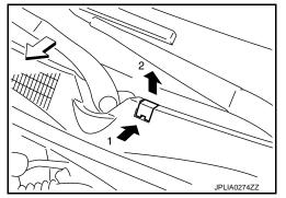
3. Remove the front washer tube from the front washer nozzle.
